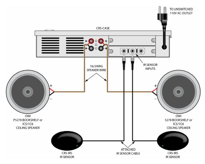
Figure 14. Typical CRS System Connections
